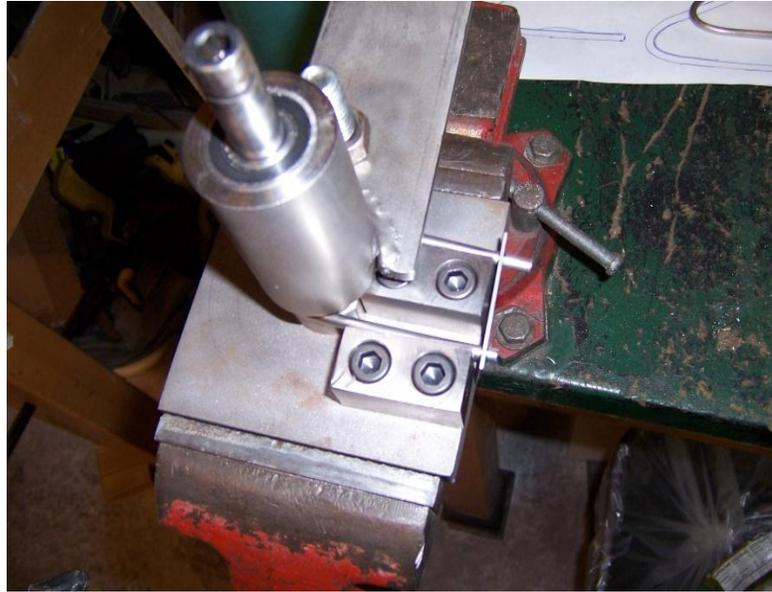
**Figure 9 Bending Jig with 316L Specimen**
